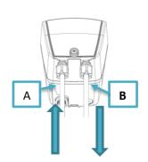
**Step 1:** Ensure there is no power to the unit, connect the suction tube from the detergent or rinse container to (A). Now connect the delivery tube from (B) to the injection point.
