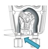
**Step 4:** Insert one end of the tube ensuring that it is slotted into the body of the enclosure as shown.
