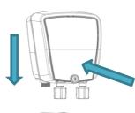
**Step 2:** Mount the unit to the wall by hooking it onto the wall bracket. As you push the unit down you should hear a click sound.
