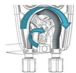
**Step 5:** Now by manually rotating the pump head, feed the tube into the unit as shown. **TIP** wse some HT5 Silicone grease on the outer of the tube to help ease the tube in and prevent any snagging.
