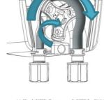
**Step 6:** Now insert the other end of the tube ensuring that it is slotted into the body of the enclosure as shown.
