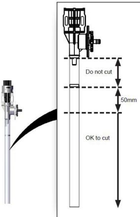
To prevent foaming, the outlet tube may need to be shortened to limit the amount of space between the bottom of the outlet tube and the bottom of the spray bottle. To do this, cut the lower section of the tube ensuring not to cut between the flood ring and outlet.
