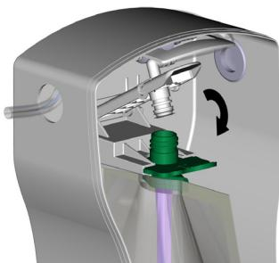
Secure the chemical concentrate pouch in place and clip plastic seal firmly on top of pouch. To change the direction of the clear PVC chemical suction tubes, unclip the angle connector in the pouch adaptor, rotate 180 degrees and click back in place.
