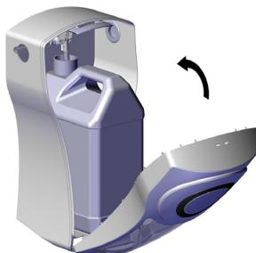
The clear PVC chemical suction tubes can go through either side of the cabinet. To change its direction, pull down gently on the angle connector, turn the tube around to the other side and clip back into place.
