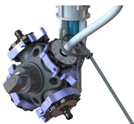
Attach clear PVC chemical suction tubes to the non-return valves to enable chemical delivery. It is recommended to cable tie both the black chemical inlet tubes and clear PVC chemical suction tubes to form a seal.
