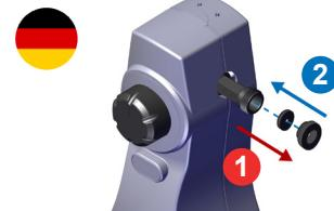
The water inlet direction must be set. This can be changed by removing the retaining pins (2.1), swapping the inlet connector with the end cap (2.2) and (2.3), replacing pins (2.4). Then re-attach the internal assembly securely to the backplate. (2.6) **FOR GERMANY & LOW FLOW VERSION ONLY**, please remove the washer and insert the restrictor as shown. Once you have inserted the restrictor, reinser the washer to the original position
