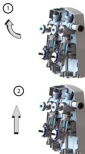
To mount the unit, first remove the cover using the key provided (1.2), then unclip the non-return valves (1.3), release the retaining clips (1.3), and remove the venturi internals (1.4).
