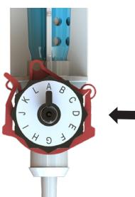
Pull the dilution clip out to the furthest position. Pull the dilution pin out to enable rotation of the letters. Select the correct dilution at the top (12:00). Return the dilution pin and clip to form a closed seal.
